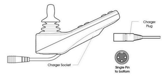
Do not exceed the maximum charging current of 12Arms. Always use an off-board charger fitted with a Neutrik NC3MX plug. Failure to observe these conditions could result in poor contact resistance in the charger connector resulting in overheating of the charger plugs. This presents a potential burn hazard for the user. PGDT accepts no liability for losses of any kind arising from failure to comply with this condition.
