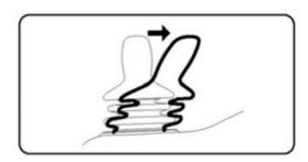
If you do not push the joystick as you switch the wheelchair on and the diagnostic screen is displayed, as in the following diagram, then the R-net has detected a problem somewhere in the wheelchair's electrical system.
