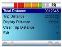
**Total Distance**: This is a value held in the Power Module and relates to the total distance driven using that Power Module.
